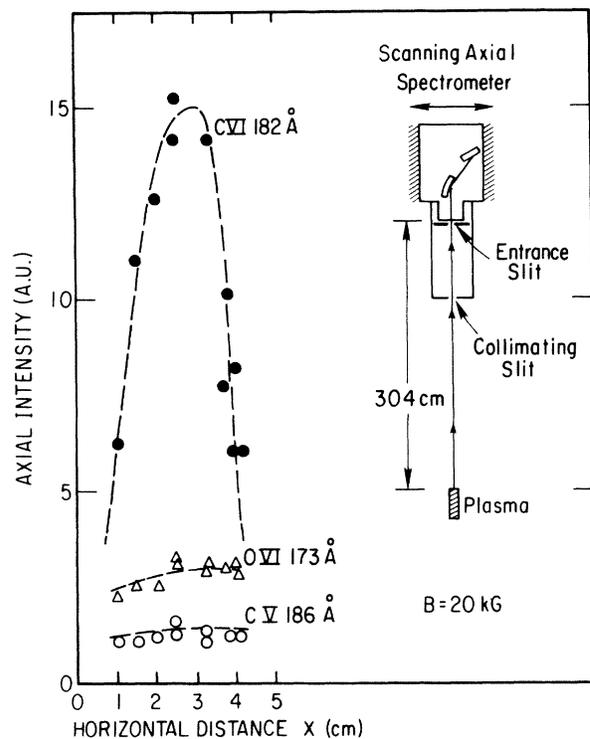
FIG. 3. Absolute divergence measurements ( $\sim 9 \text{ mrad}$ ) of the 182-Å lasing radiation for a magnetic field  $B = 20 \text{ kG}$ . For comparison the intensities of nonlasing lines O VI 173 Å and C V 186 Å are shown, recorded simultaneously with the 182-Å line.
