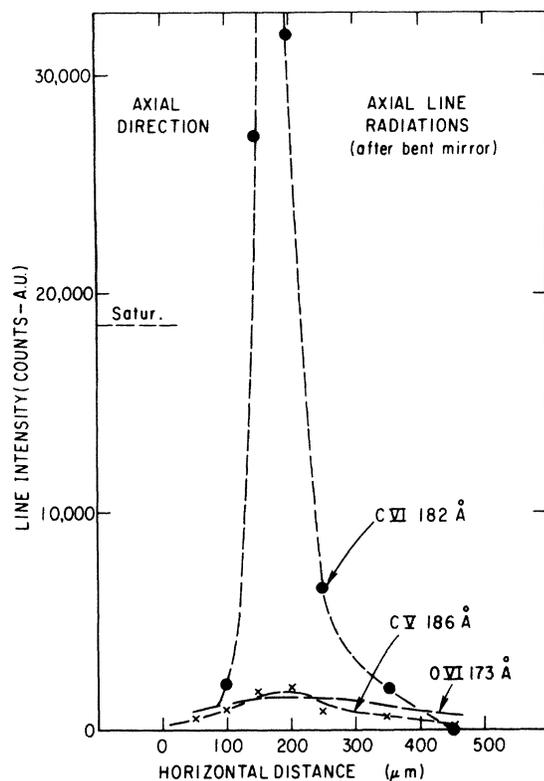
FIG. 2. Transverse scan of C VI 182-Å, C V 186-Å, and O VI 173-Å emission showing a strong central peak for the C VI 182-Å stimulated emission. "Satur." indicates the level above which the detector is saturated. Intensities above this level were obtained by comparing the nonsaturated regions of the 182-Å spectral profiles.
