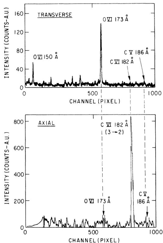
FIG. 1. Transverse and axial spectra in the region near 182-Å from a carbon-disk target with four carbon blades. The laser energy was 500 J.
