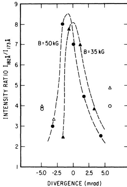
FIG. 4. Divergence measurements ( $\sim 5$  mrad) of the 182-Å radiation (relative to the O VI 173-Å line) for  $B=35$  and 50 kG.
