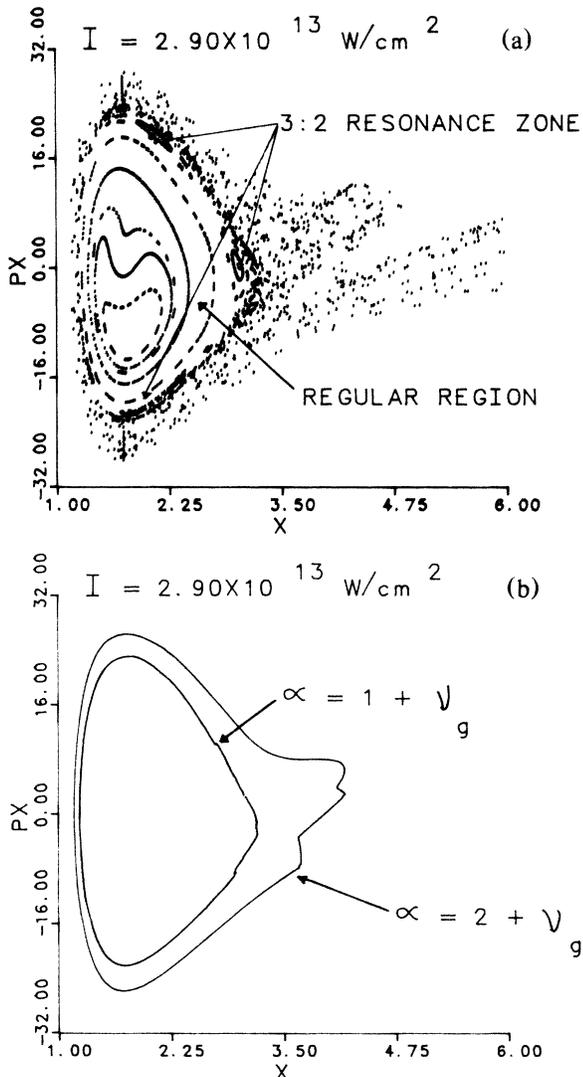
FIG. 1. (a) The  $x$ - $p$  surface of section for the Hamiltonian describing the interaction between an anharmonic oscillator and an intense radiation field. (b) Phase-space representation of the cantori resulting from the breakup of tori with winding numbers equal to 1 and 2 plus the golden mean.
