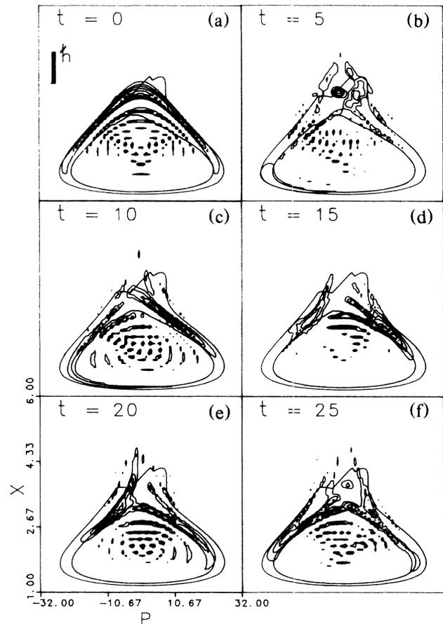
FIG. 2. Contour plots (positive contours only) for the Wigner transform of a nonstationary state for an anharmonic oscillator evolving in response to the radiation field after (a) 0, (b) 5, (c) 10, (d) 15, (e) 20, and (f) 25 field periods ( $\tau = 0.054$  ps). The cantori shown in Fig. 1(b) are also shown in each of the diagrams (a)–(f). A box indicating the size of  $\hbar$  is shown in (a).
