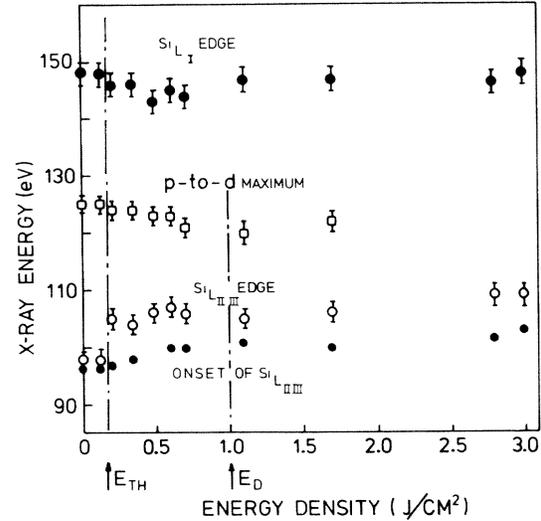
FIG. 2. Onset of the Si- $L_{II,III}$  absorption, Si- $L_{II,III}$  and Si- $L_I$  (effective) edges, and  $p$ -to- $d$  maxima as functions of the laser energy density. ( $E_{th}$  = annealing threshold;  $E_d$  = damage threshold.)
