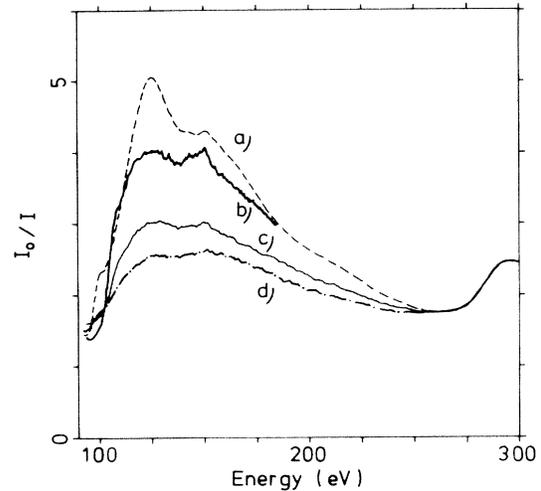
FIG. 3. Time evolution of the x-ray absorption spectra of short-lived *l*-Si produced by irradiation at  $0.30 \pm 0.04 \text{ J/cm}^2$ . Delay times are (b) 12 ns, (c) 30 ns, and (d) 60 ns. Spectrum (a) is a reference, recorded without laser irradiation.
