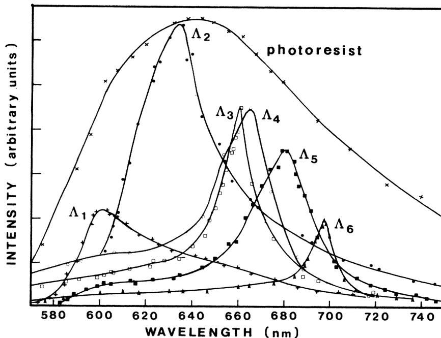
FIG. 2. Photoresist fluorescence spectrum and Ag-air interface SP radiative emission spectra for gratings having periods (in nanometers)  $\Lambda_1 = 760$ ,  $\Lambda_2 = 814$ ,  $\Lambda_3 = 898$ ,  $\Lambda_4 = 900$ ,  $\Lambda_5 = 926$ ,  $\Lambda_6 = 976$ .
