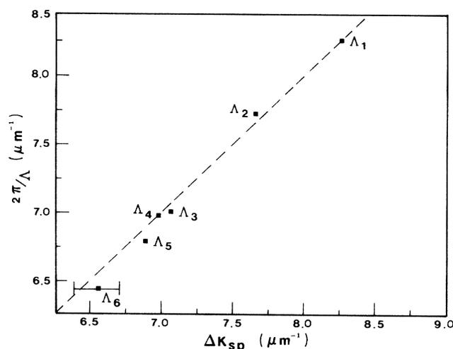
FIG. 4. Comparison of grating constant  $2\pi/\Lambda_i$  with the difference  $\Delta k_{sp}$  between surface plasmons on opposite sides of grating  $\Lambda_i$  and at the same peak emission wavelength  $\lambda_i$ . Horizontal error bars associated with grating  $\Lambda_6$  represent an estimated  $\pm 3\%$  error in the measured values of  $\Delta k_{sp}$  and are the same size for all six points.
