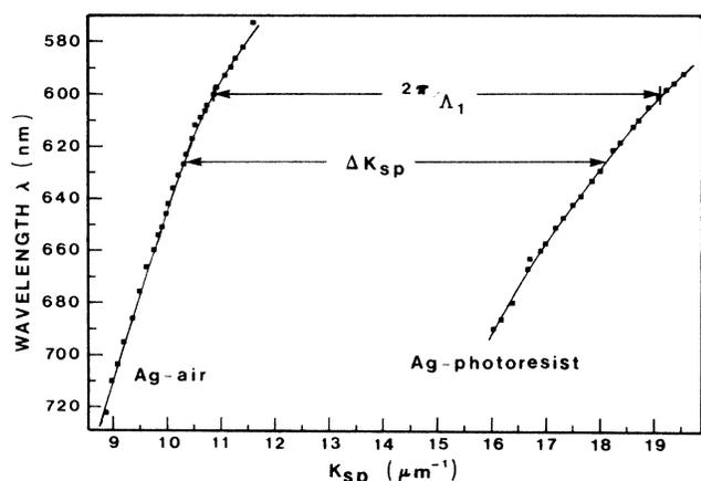
FIG. 3. Experimental dispersion curves for surface plasmons at the Ag-air and Ag-photoresist corrugated interfaces with  $\Lambda_1 = 760$  nm. The grating constant  $2\pi/\Lambda_1$  phase matches the two SP at  $\lambda_1 = 600$  nm, the peak emission wavelength for the grating having period  $\Lambda_1$ .
