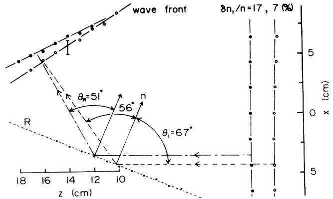
FIG. 3. Typical examples of the wave front of incident solitons and reflected waves. The incident soliton amplitude refers to  $\delta n/n = 7\%$  (open circles) and  $17\%$  (filled circles) and both of the incident angles are  $67^\circ$ . R is a reflector.
