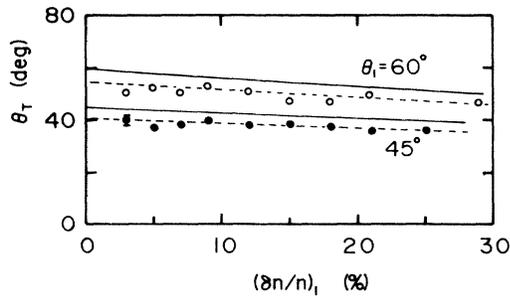
FIG. 5. Refraction angle  $\theta_T$  vs incident wave amplitude for constant incident angle  $\theta_I$ . Solid lines are calculated from Eq. (2).
