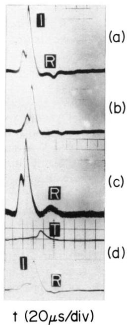
FIG. 2. Typical examples of the wave form. (a) Reflection of negative pulse:  $V_{\text{bias}} = -25$  V (floating), (b) no reflections:  $V_{\text{bias}} = -150$  V, (c) reflection of positive pulse:  $V_{\text{bias}} = -500$  V, and (d) transmitted wave:  $V_{\text{bias}} = -50$  V.
