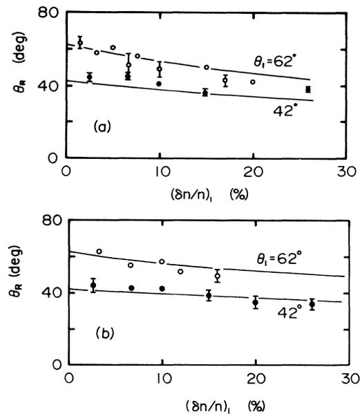
FIG. 4. Reflection angles  $\theta_R$  vs incident wave amplitude for constant incident angle  $\theta_I$ . The reflected wave has negative polarity in (a) and positive polarity in (b). Solid lines are calculated from Eq. (2).
