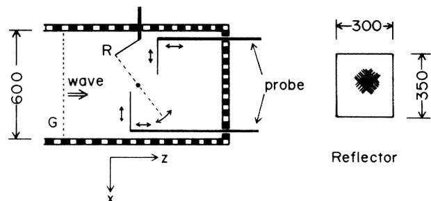
FIG. 1. Schematics of the experimental apparatus. G is a separation grid for exciting solitons and R is a metallic mesh reflector (6 mesh/cm).
