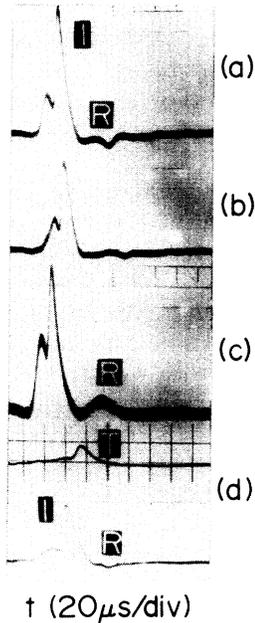
FIG. 2. Typical examples of the wave form. (a) Reflection of negative pulse:  $V_{\text{bias}} = -25$  V (floating), (b) no reflections:  $V_{\text{bias}} = -150$  V, (c) reflection of positive pulse:  $V_{\text{bias}} = -500$  V, and (d) transmitted wave:  $V_{\text{bias}} = -50$  V.
