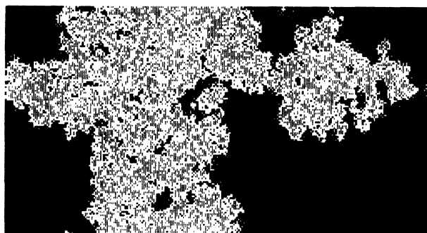
FIG. 5. With y_{\text{CO}}=0.527 , slightly above y_2 , CO poisoning is slowly occurring (non-steady-state).
