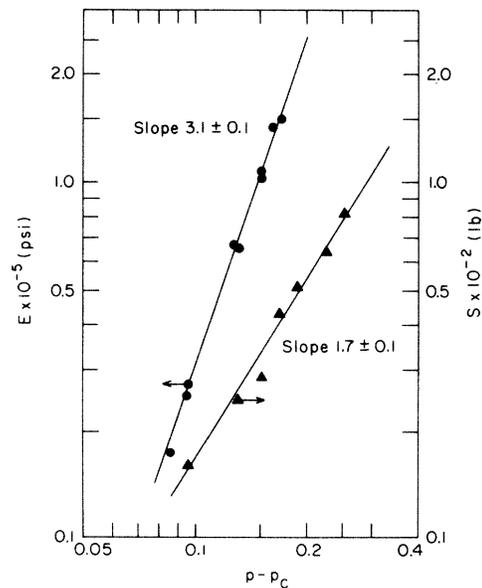
FIG. 3. Double logarithmic plot of  $E$  and  $S$  vs  $p - p_c$ ,  $p_c = 0.63$ .
