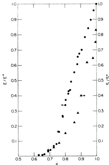
FIG. 2. Normalized Young's modulus,  $E/E^0$ , and fracture stress,  $S/S^0$ , as functions of  $p$ .
