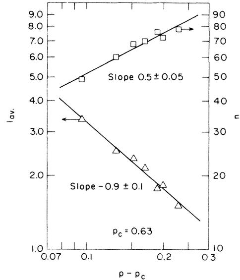
FIG. 4. Double logarithmic plot of  $l_{av}$  and the number of the cracks,  $n$ , vs  $p - p_c$ ;  $p_c = 0.63$ .
