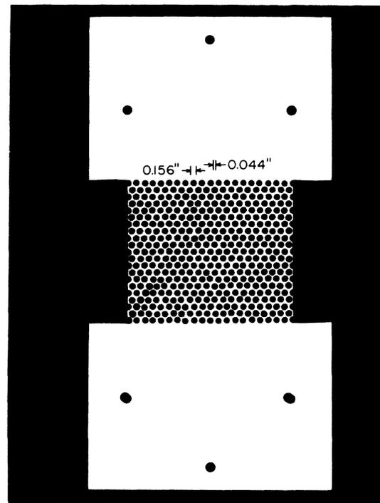
FIG. 1. The configuration of the 2D triangular network. The ligaments connecting the voids are randomly cut forming cracks as described in the text.
