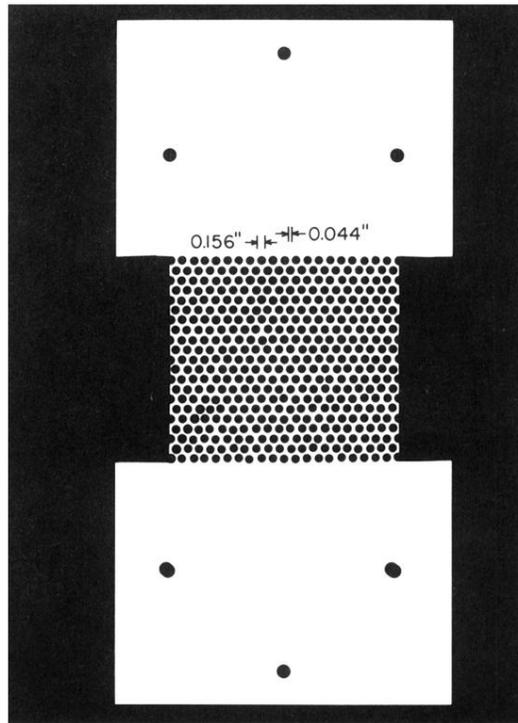
FIG. 1. The configuration of the 2D triangular network. The ligaments connecting the voids are randomly cut forming cracks as described in the text.
