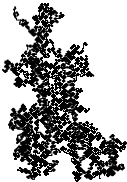
FIG. 3. Typical cluster generated by poisoned Eden growth with an equal mixture of two- and four-functional monomers. The cluster contains 6400 sites. The plus signs represent growth sites. The surface fractal dimension, D_s , obtained from the radius dependence of the perimeter is 1.5 \pm 0.1 , whereas the mass fractal dimension, D , obtained from the mass dependence of the radius, is 2.0 \pm 0.1 .
