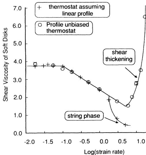
FIG. 1. Viscosity as a function of the base-10 logarithm of the shear rate for a two-dimensional soft-disk fluid. The standard NEMD algorithm leads to the formation of a string phase at high shear rates. This phase's existence is brought about by the assumption of a linear velocity profile in the formulation of the thermostat. This assumption is incorrect at high Reynolds numbers.
