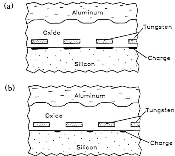
FIG. 2. Q1D charge-confinement schemes. (a) Subgrating confinement, where the upper gate is fixed and the grating controls the electron density. (b) Gap confinement, where the upper electrode is the control.
