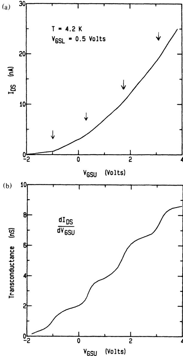
FIG. 3.  $I_{DS}$ - $V_{UGS}$  (source-drain current vs upper gate bias) data for a Q1D device operated in the gap inversion mode at 1.2 K. (a) Normal  $I_{DS}$  vs  $V_{UGS}$ , and (b) derivative ( $\partial I_{DS}/\partial V_{UGS}$ ) vs  $V_{UGS}$ .
