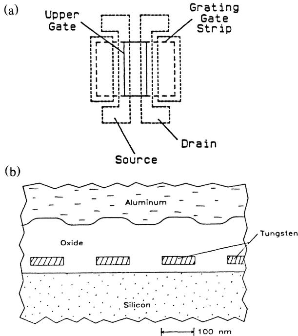
FIG. 1. Q1D grating-gate device structure. (a) Schematic of the device layout, illustrating the  $n^+$  source and drain, grating-gate strip, upper gate, and contact areas. (b) Channel cross section showing the dual, stacked-gate configuration with  $0.2\text{-}\mu\text{m}$ -period W grating.
