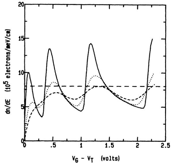
FIG. 4. Plots of the effective density of states,  $\bar{g}_1$ , in a Q1D conductor showing the decrease in modulation amplitude with increasing temperature. System modeled is a square well of width 50 nm at  $T = 1.2, 4.2,$  and  $8$  K. Dashed line is the equivalent 2D approximation for the same channel width (i.e.,  $g_2 W$ ).
