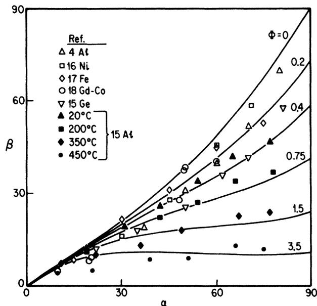
FIG. 3. Column orientation as a function of incident beam angle; data from Refs. 4 and 15–18. Four substrate temperatures are plotted for aluminum, from Ref. 15.
