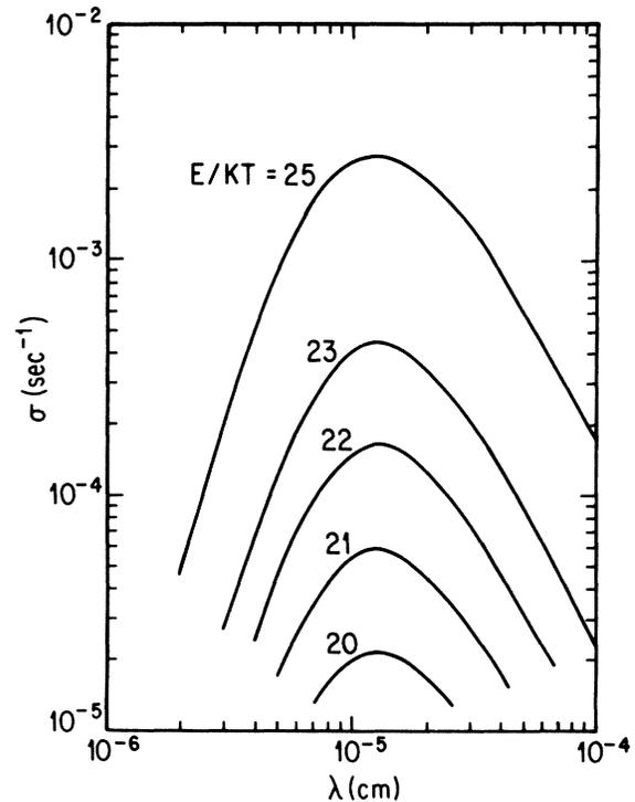
FIG. 2. Growth rate as a function of column wavelength. The curves are for  $J = 10 \text{ \AA}/\text{sec}$ ,  $\langle x^2 \rangle = 4 \times 10^4 \text{ \AA}^2$ , and  $\alpha = 30^\circ$ ,  $a = 4.05 \text{ \AA}$ , and  $\nu = 10^{13}/\text{sec}$ .
