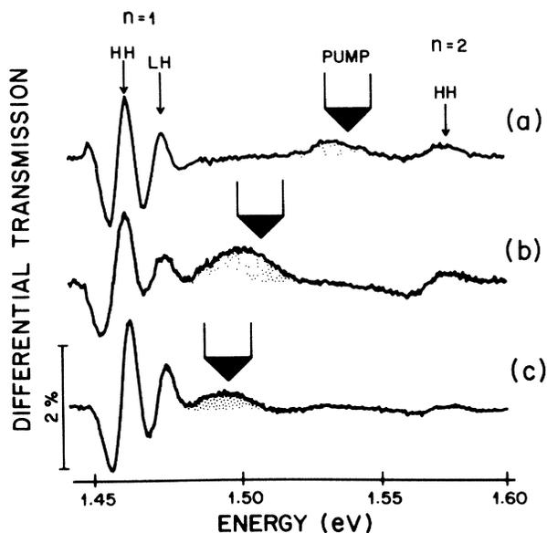
FIG. 1. Differential transmission spectra at nominally zero delay. The three spectra correspond to excitation by 100-fs pulses centered at (a) 1.537 eV, (b) 1.509 eV, and (c) 1.496 eV. The spectral width of the exciting pulse is  $\sim 20$  meV. HH and LH refer to heavy-hole and light-hole excitons, respectively.
