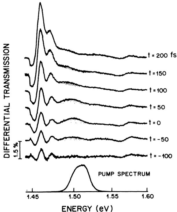
FIG. 2. Differential transmission spectra for a pump centered at 1.509 eV and observed at 50 fs intervals between  $t = -100$  fs and  $t = +200$  fs. The spectra have been displaced vertically for clarity. The pump spectrum is shown at the bottom of the figure. Various features are discussed in the text.
