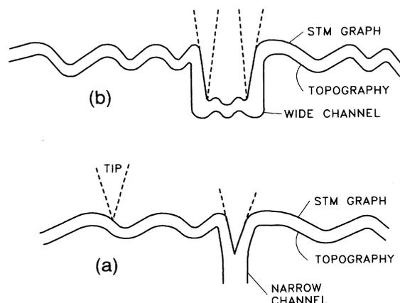
FIG. 3. A schematic illustration of the scanning of the tip across a trench site for (a) a narrow trench and (b) a wide trench with respect to the tip dimensions. Both topography and the corresponding STM graph are shown.
