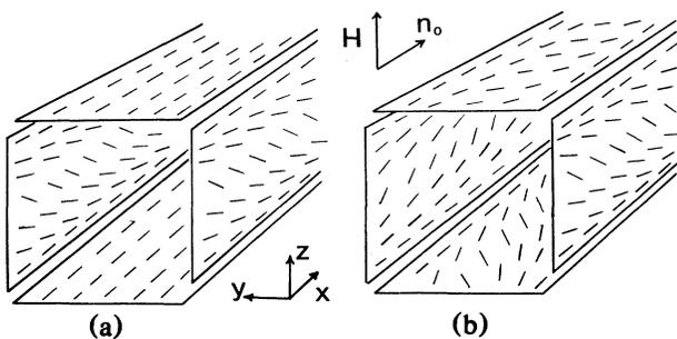
FIG. 2. Schematic representation of (a) the uniform splay-Fréedericksz distortion, and (b) the periodic splay-twist distortion.
