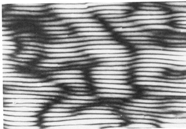
FIG. 1. Polarized-light photomicrograph of the periodic splay-twist distortion in PBG. The distance between two dark bands is  $32.5 \mu\text{m}$ . The field is perpendicular to the plane of the sample, and the unperturbed director is parallel to the stripes.
