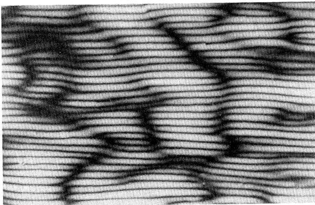
FIG. 1. Polarized-light photomicrograph of the periodic splay-twist distortion in PBG. The distance between two dark bands is 32.5  $\mu\text{m}$ . The field is perpendicular to the plane of the sample, and the unperturbed director is parallel to the stripes.
