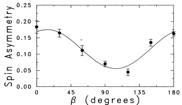
FIG. 3. Spin asymmetry  $(N_{\uparrow} - N_{\downarrow}) / (N_{\uparrow} + N_{\downarrow})$  in superelastic scattering vs laser polarization angle  $\beta$ . The scattering angle is  $-30^\circ$ .  $\beta = 0$  corresponds to the incident electron direction. The curve is a least-squares fit of the function  $A + B \cos(2\beta + C)$ . The parameters  $A$ ,  $B$ , and  $C$  have the values  $0.115 \pm 0.006$ ,  $0.060 \pm 0.008$ , and  $-28^\circ \pm 9^\circ$ .
