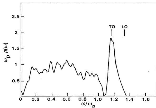
FIG. 3. Density of states with the peak frequencies in the transverse and longitudinal responses in Fig. 2 indicated by TO and LO. The resolution is  $0.03\omega_p$ .
