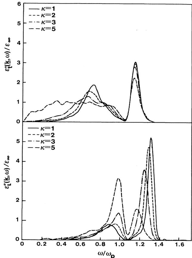
FIG. 1. Imaginary parts of the transverse and longitudinal dielectric functions for various wave vectors  $\mathbf{k} = 2\pi(0, 0, \kappa)/L$ . The resolution is  $0.05\omega_p$ .
