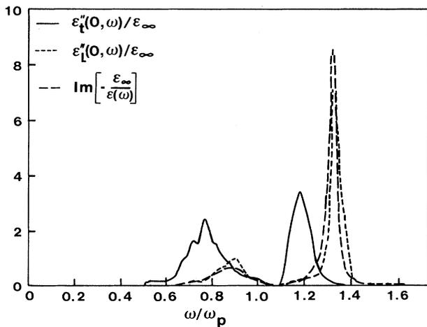
FIG. 2. Imaginary parts of the long-wavelength limit of the transverse and longitudinal dielectric functions and the loss function  $\text{Im}[-\epsilon_\infty/\epsilon(\omega)]$ . The resolution is  $0.03\omega_p$ .
