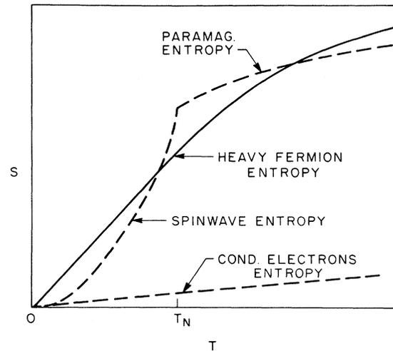
FIG. 2. A schematic diagram useful for arguing the condition under which a heavy-fermion mass is obtained—see text. The dashed lines refer to the entropy contribution in a typical rare-earth metal or metallic compound, and the solid line to the entropy in a heavy-fermion material. The phonon contribution to the entropy has been ignored.
