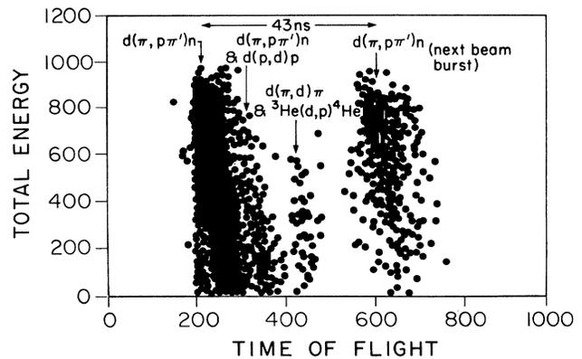
FIG. 2. Time of flight at D vs the total energy in P after the polarimeter showing the separation of  $(d,p)$  events from background. The scales drawn are in channel numbers. The separation of the beam bursts is 43 ns as indicated.
