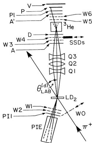
FIG. 1. Experimental configuration at TRIUMF. The scattered pions were detected in wire chambers (W1,W2) and scintillators (PII,PIE). The recoil deuterons were focused by the quadrupole triplet onto the polarimeter consisting of a  $^3\text{He}$ -gas cell surrounded by wire chambers (W3,W4,W5,W6), scintillators (D,P1,P,V), absorbers (A,A'), and retractable solid-state detectors (SSD's).
