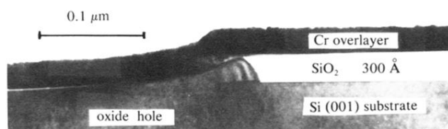
FIG. 2. Cross-sectional TEM micrograph for ultrahigh-vacuum annealing of a 300-Å-SiO 2 layer on Si(001) until about 15% of the surface is oxide free. Before preparation of the sample for cross-sectional TEM analysis, it was covered with \sim 300 Å of Cr to provide a contrasting layer between the SiO 2 and the glue used in the sample preparation.
