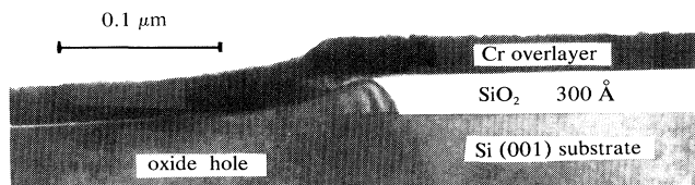
FIG. 2. Cross-sectional TEM micrograph for ultrahigh-vacuum annealing of a 300-Å-SiO 2 layer on Si(001) until about 15% of the surface is oxide free. Before preparation of the sample for cross-sectional TEM analysis, it was covered with \sim 300 Å of Cr to provide a contrasting layer between the SiO 2 and the glue used in the sample preparation.
