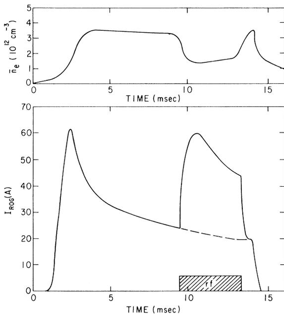
FIG. 2. Circulating current  $I_{rog}$ , and density  $\bar{n}_e$ , during the main discharge. The 18-MHz rf power is on for a duration of 5 msec in alternate discharges. The discharge without rf is indicated by the dashed curve. The injected electron beam produces the current that circulates normally, and FWCD augments that current when rf power is applied. The discharges are highly repeatable.
