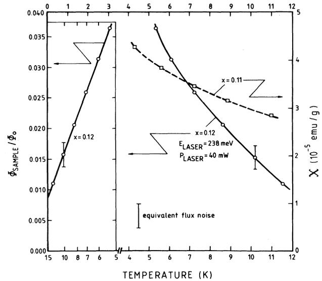
FIG. 2. Photomagnetization in an open-gap  $\text{Hg}_{1-x}\text{Mn}_x\text{Te}$  sample vs temperature. For comparison, the low-field magnetic susceptibility (Ref. 8) of  $\text{Hg}_{0.89}\text{Mn}_{0.11}\text{Te}$  with similar chemical composition is shown. The photomagnetization effect is inversely proportional to the temperature (see inset).
