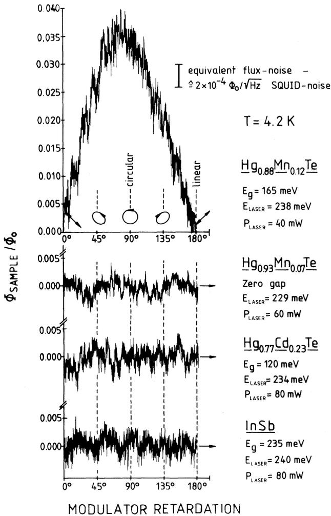
FIG. 1. Magnetic flux in the pickup coil proportional to the magnetization of various semiconductor samples vs the degree of circular polarization of the CO-laser radiation. Only in the open-gap diluted magnetic semiconductor  $\text{Hg}_{0.88}\text{Mn}_{0.12}\text{Te}$  is the photomagnetization observed.
