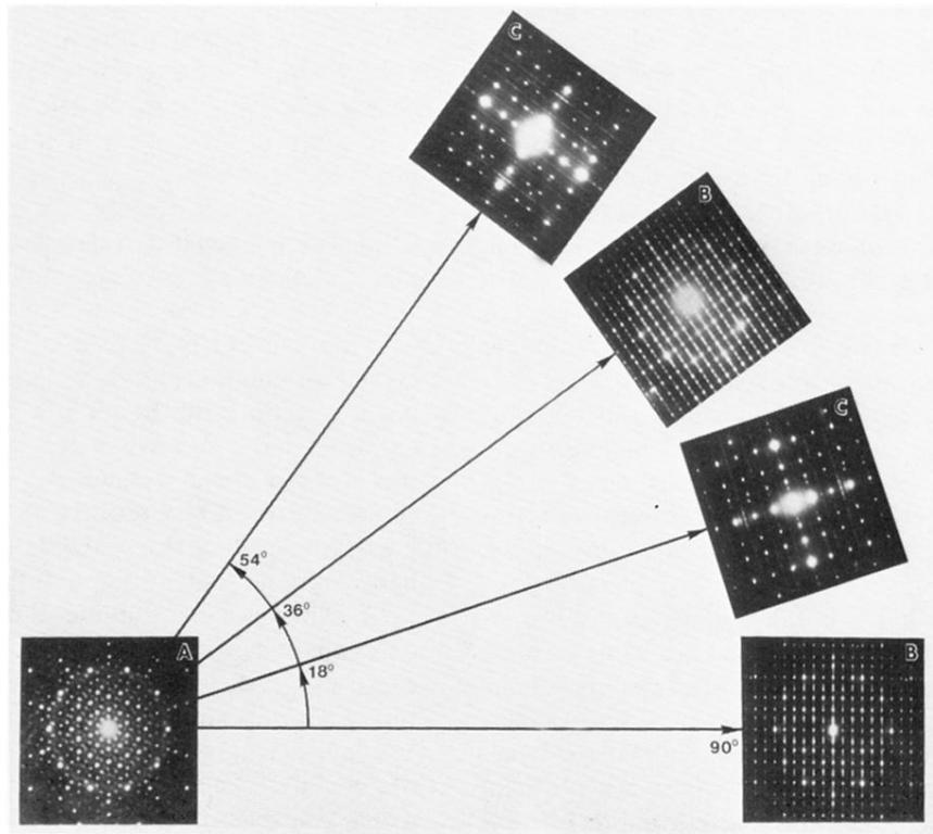
FIG. 1. Selected-area electron diffraction patterns taken from a single grain of the decagonal phase.
