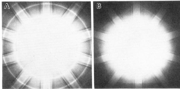
FIG. 2. Convergent-beam electron diffraction patterns from the (a) decagonal and the (b) icosahedral phases. Whole-pattern symmetries are 10 (or  $10mm$ ) and  $\bar{5}m$ , respectively.
