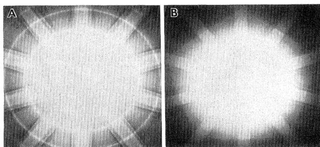
FIG. 2. Convergent-beam electron diffraction patterns from the (a) decagonal and the (b) icosahedral phases. Whole-pattern symmetries are 10 (or  $10mm$ ) and  $\bar{5}m$ , respectively.
