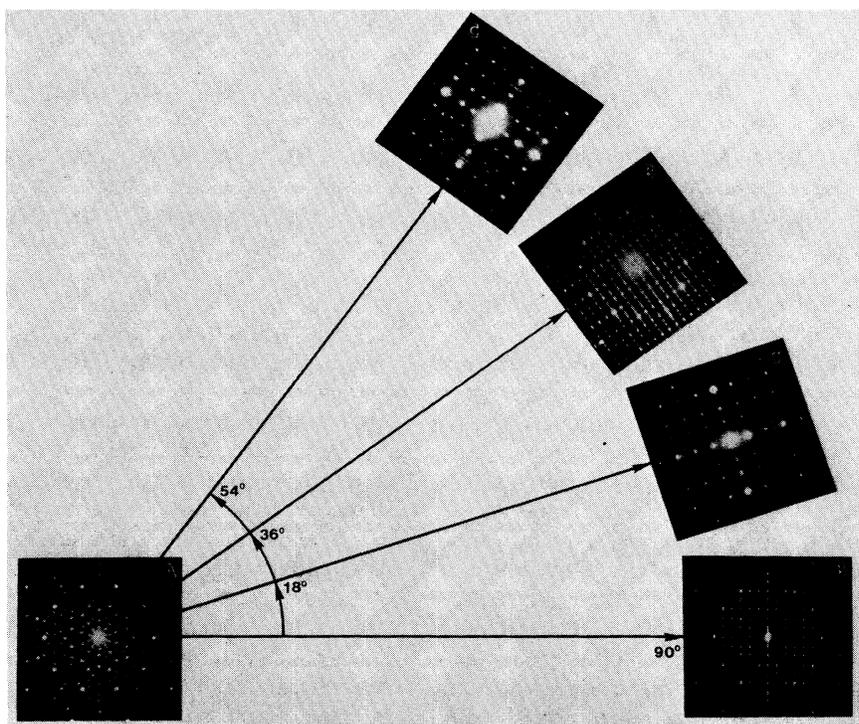
FIG. 1. Selected-area electron diffraction patterns taken from a single grain of the decagonal phase.
