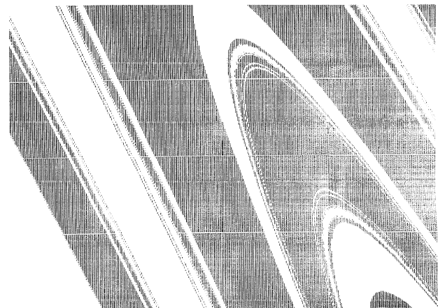
FIG. 3. Composite photograph of finer scale enlargement of Fig. 2 basin boundary for 160 \times 10^3 initial conditions, f = 0.1 , \omega = 0.833 , \gamma = 0.15 , -0.375 \leq x_0 \leq -0.275 , 0.045 \leq v_0 \leq 0.075 .
