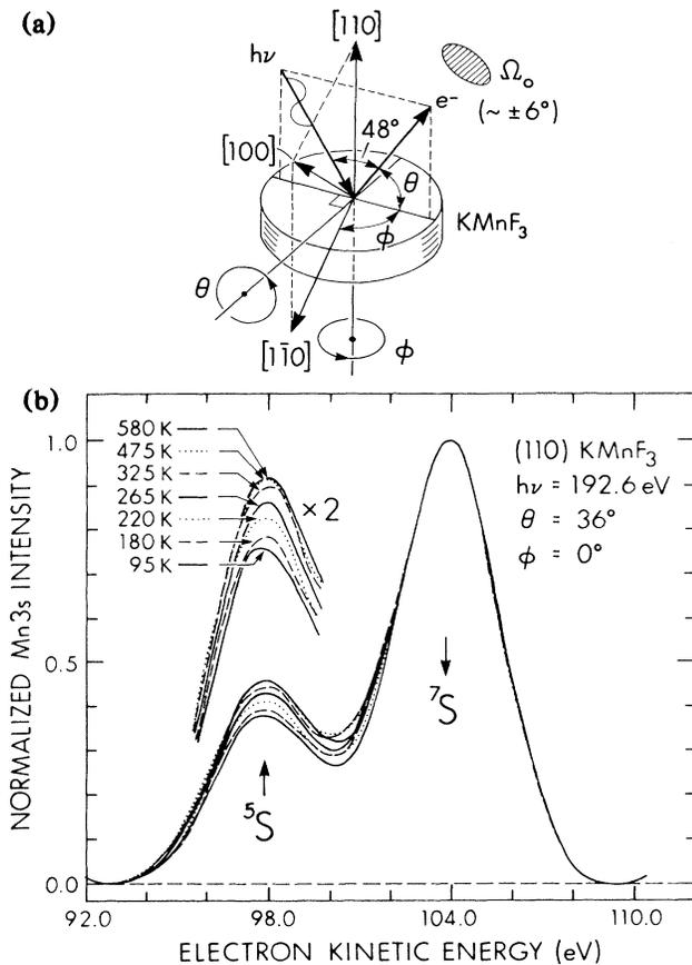
FIG. 1. (a) Experimental geometry for photoemission from a (110) surface of  $\text{KMnF}_3$ , with pertinent angles defined. The radiation is unpolarized. (b) Mn 3s spectra at several temperatures, with normalization to the  $7S$  or "spin-down" peak. Mo  $M\zeta$  radiation at 192.6 eV is used for excitation. Emission is along  $\theta = 36^\circ$ ,  $\phi = 0^\circ$ .
