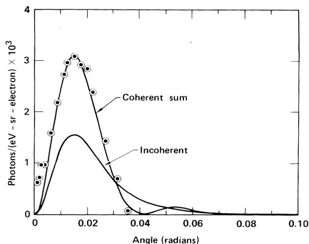
FIG. 3. Comparison of the TR angular distribution for 1- $\mu$ m-thick beryllium foils calculated with [see Eq. (4)] and without the effects of coherent interference between the two surfaces of each foil. The measured intensity and angular distribution clearly demonstrate interference between the two foil surfaces.
