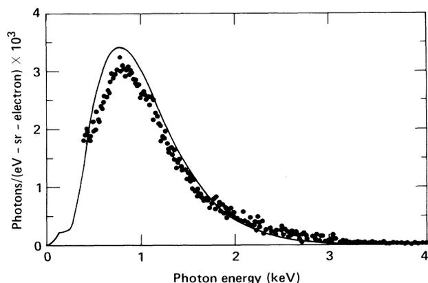
FIG. 2. Comparison of the measured and calculated TR spectra at 15 mrad for 25-MeV electrons incident on a stack of eighteen 1- $\mu$ m-thick beryllium foils. The calculation (solid curve) includes the spectral dependence of the detector efficiency but ignores unobservable interference between foils in the stack.
