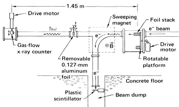
FIG. 1. Experimental apparatus for measuring photon spectra and angular distributions from various stacks of foils. The electrons enter from the right, pass through the foil stack, and are dumped into a deep hole in the floor. The photons travel 145 cm from the stack to a translatable gas-proportional detector. To measure the background in the room, a 0.127-mm-thick aluminum foil is inserted to block soft x rays.
