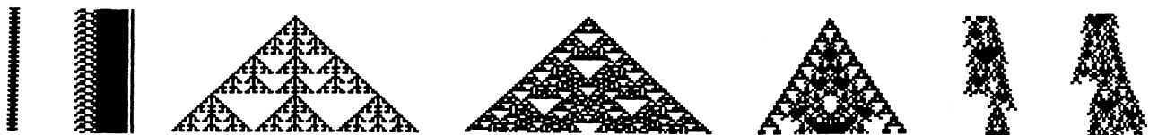
FIG. 1. Seven examples of patterns generated by repeated application of various simple cellular automaton rules. The last four are probably computationally irreducible, and can be found only by direct simulation.
