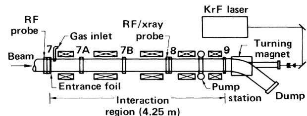
FIG. 1. Experimental configuration on the experimental test accelerator. The station numbers refer to resistive-wall current monitors. Solenoidal transport magnets are shown in cross section.
