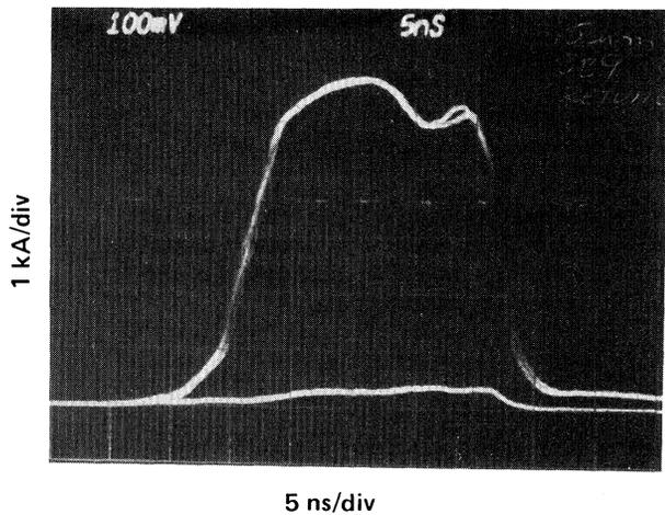
FIG. 2. Beam current at monitor 9 with the laser channel present (upper traces) and with the laser off (lower traces). All solenoidal magnets were off, 0.5-mT benzene pressure, small laser beam ( $a \approx 0.26$  cm),  $0.41\text{-J cm}^{-2}$  laser fluence,  $n_i \approx 5.6 \times 10^{11} \text{ cm}^{-3}$ .
