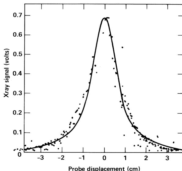
FIG. 5. X-ray wire-probe data (points) and fitted beam profile (line) at monitor 7B (2.4 m from entrance foil) for large-channel beam transport,  $a \approx 0.83$  cm,  $P = 1$  mT. Each point is one beam pulse. The curve parameters are  $x = 1.15$ ,  $\mu = 5$ .
