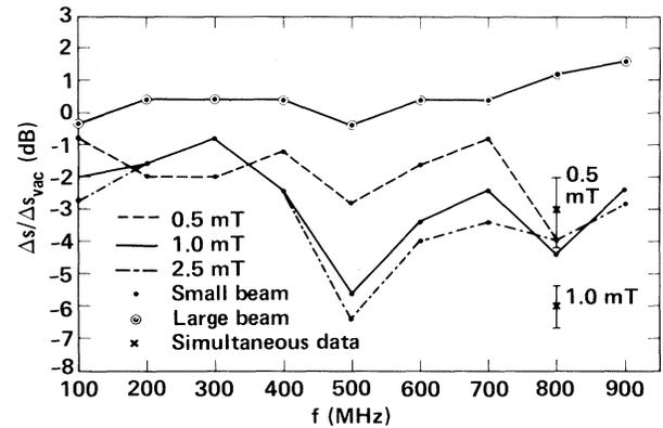
FIG. 3. Laser-channel damping of low-frequency (sweep) and high-frequency (beam-breakup) beam motion. The time-averaged rf-probe signals were measured with a spectrum analyzer and are normalized to vacuum (solenoidal) transport values.  $\Delta s$  refers to the ratio of the downstream-to-upstream signal averages. The two points with error bars were obtained by simultaneous upstream and downstream measurements at 800 MHz of the deliberately excited beam-breakup mode.
