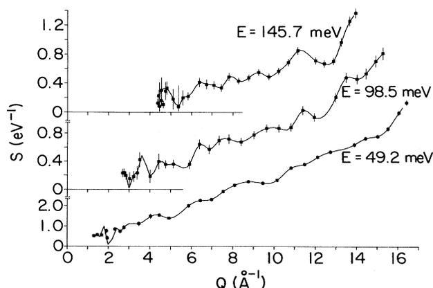
FIG. 3.  $Q$  variation of  $S(Q, E)$  for  $\alpha$ -SiO<sub>2</sub> at  $E = 49.2$ , 98.5, and 145.7 meV. The solid curves represent cubic spline fits through the data, taking account of the statistical errors indicated by the bars on each data point.
