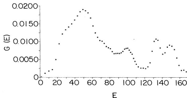
FIG. 2. One-phonon density of states  $g_i(E/\hbar)$  for  $\alpha\text{-SiO}_2$ .
