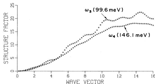
FIG. 4.  $S^{(1)}(Q, E)$  for the  $\omega_3$  and  $\omega_4$  modes of the Sen-Thorpe model (Ref. 10).
