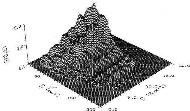
FIG. 1. Scattering function of  $\alpha\text{-SiO}_2$  at 33 K.
