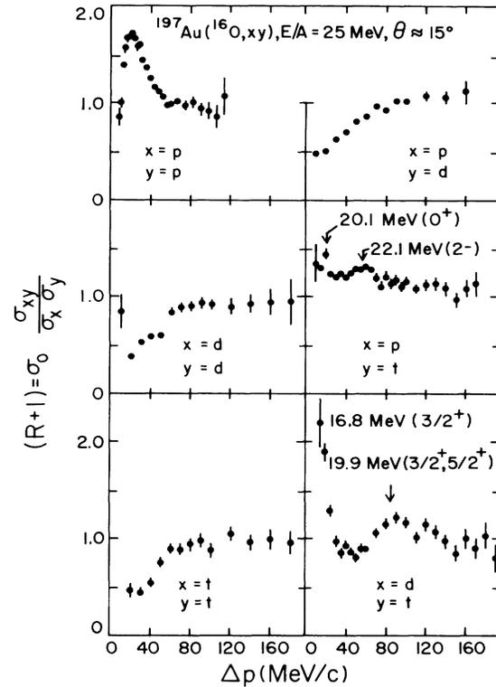
FIG. 1. Experimental correlation functions,  $1 + R(\Delta p)$ , plotted as a function of the momentum of relative motion. The locations of several known particle-unstable resonances are indicated by arrows. The errors are purely statistical.
