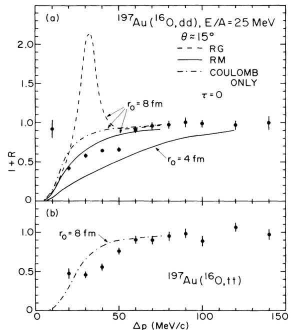
FIG. 2. (a) Comparison of  $d$ - $d$  correlation function data with calculations based on phase shifts of Refs. 16 (RM) and 17 (RG). The dot-dashed curve neglects the nuclear part of the potential. (b) Comparison of  $t$ - $t$  correlation function data with a calculation using only the Coulomb part of the potential. The radius parameter  $r_0$  is indicated. The experimental correlation functions were normalized to  $R(\Delta p) = 0$  at large relative momenta.
