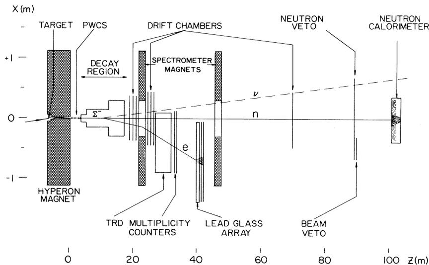
FIG. 2. Plan view of the apparatus; note that the  $x$  and  $z$  scales are different. Typical particle trajectories are also shown. The incident proton beam corresponds to a positive targeting angle.
