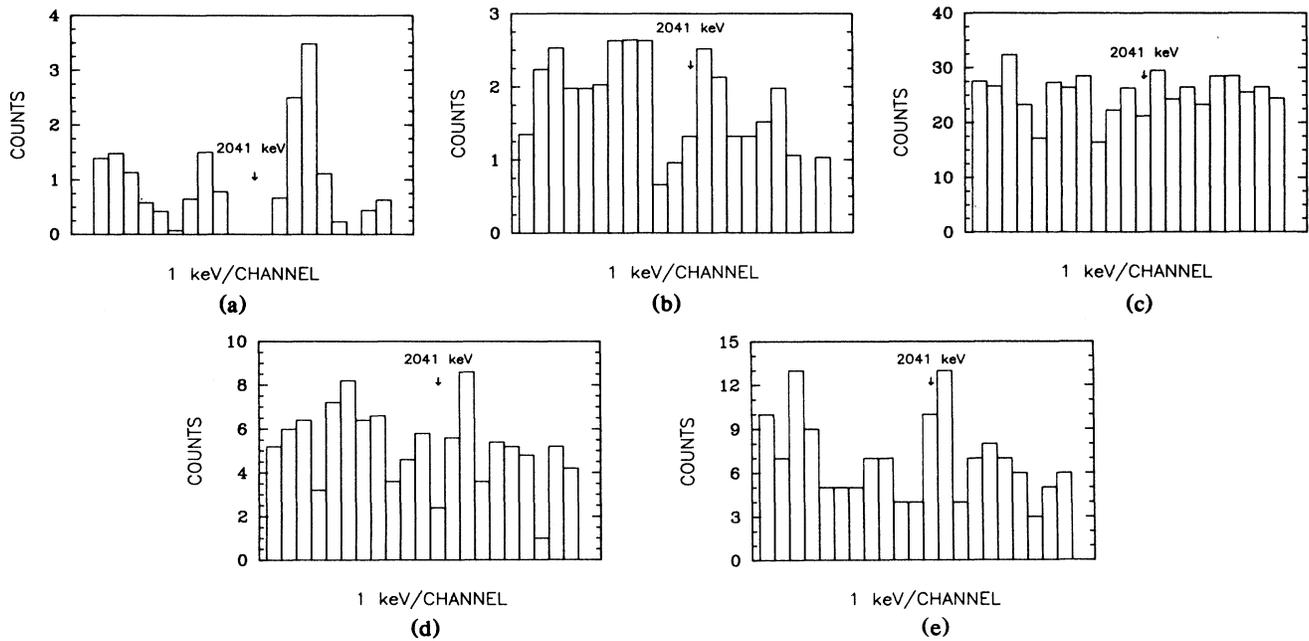
FIG. 2. Spectra from the four recent experimental searches for the neutrinoless  $\beta^-\beta^-$ -decay of  $^{76}\text{Ge}$ . All spectra are gain shifted to 1 keV per channel. (a) Present work,  $Nt = 1.88 \times 10^{23}$  yr; (b) Ref. 3, detector 2,  $Nt = 2.64 \times 10^{23}$  yr; (c) Ref. 3, detector 1,  $Nt = 6.77 \times 10^{23}$  yr; (d) Ref. 4,  $Nt = 0.94 \times 10^{23}$  yr; (e) Ref. 5,  $Nt = 1.21 \times 10^{23}$  yr.
