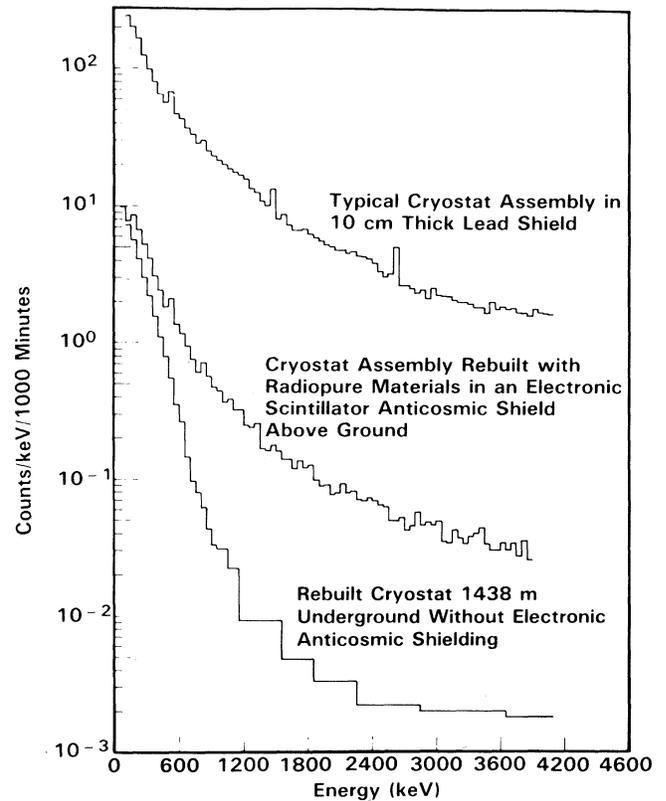
FIG. 1. Background spectra for the 135-cm<sup>3</sup> prototype Ge spectrometer in three different cryostat and shielding configurations.
