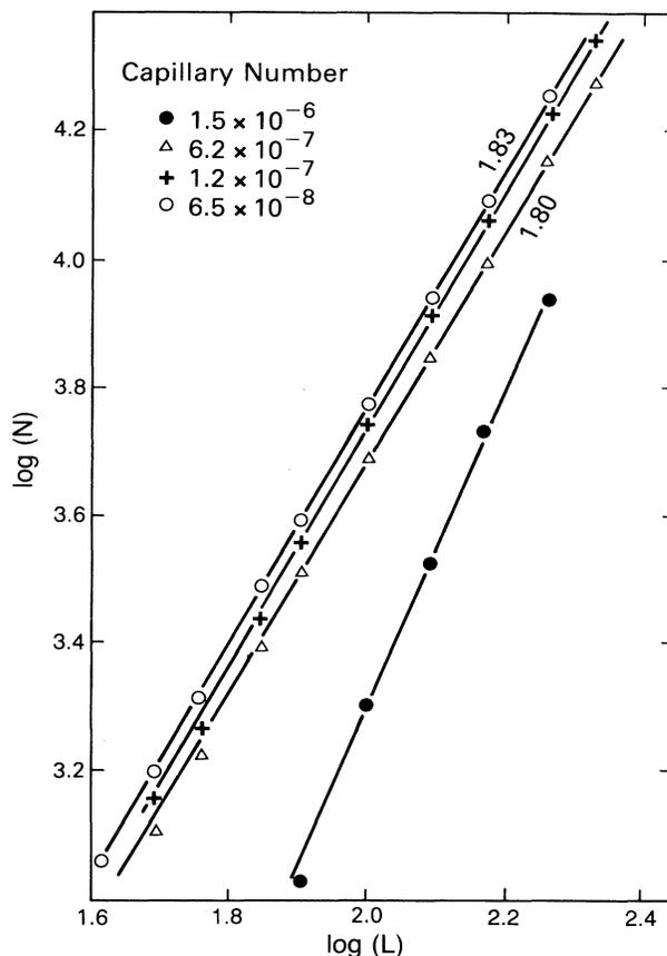
FIG. 4. Number of filled ducts vs size of the  $L \times L$  square for different capillary numbers. The slopes 1.83 and 1.80 are least-squares fit to the data. (The data for  $N_{ca} = 3.3 \times 10^{-8}$  are exactly the same as for  $N_{ca} = 6.5 \times 10^{-8}$  and are not shown in this figure.)
