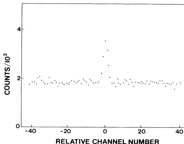
FIG. 2. A typical time-correlation spectrum after subtraction of the spectrum obtained with the metastable component of the beam quenched. Polarizer plates are removed. Time delay per channel is 0.8 ns. Total collection time is 21.5 h. Singles rate with metastables present (quenched) is about  $1.55 \times 10^4 \text{ s}^{-1}$  ( $0.85 \times 10^4 \text{ s}^{-1}$ ). True two-photon coincidence rate is  $490 \text{ h}^{-1}$ .
