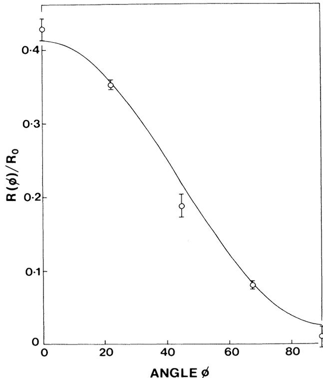
FIG. 3. Coincidence signal as a function of the angle  $\phi$  between the transmission axes of the polarizers, relative to  $R_0$ , the coincidence signal with the polarizer plates removed. The solid curve represents the QM prediction using the median values for  $\epsilon_M$  and  $\epsilon_m$ .
