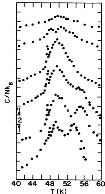
FIG. 1. Heat-capacity scans of Ar on graphite at coverages (from bottom to top)  $n = 0.175$ ,  $n = 0.572$ ,  $n = 0.717$ ,  $n = 0.872$ ,  $n = 1.043$ , and  $n = 1.068$ . For the sake of clarity, not all data points are shown.
