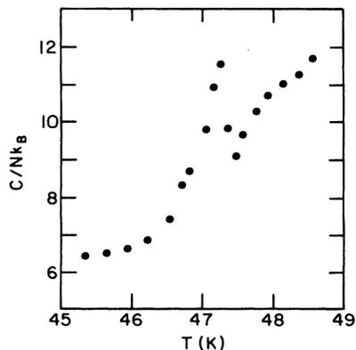
FIG. 2. Expanded view of the sharp heat-capacity peak at  $n = 0.717$ .
