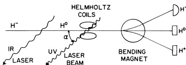
FIG. 1. Schematic diagram of the apparatus. The YAlG fundamental laser beam photodetaches  $H^-$  to produce  $H^0$ , which is then excited in the center of a Helmholtz coil by the YAlG fourth harmonic at angle  $\alpha$  with respect to the beam axis. When  $\alpha$  is tuned to match a Stark resonance, the excited atom ionizes in the coil or in the 3.6-kG bending magnet. The product  $H^+$  is deflected up to 11 mrad into a detector 2.7 m downstream.
