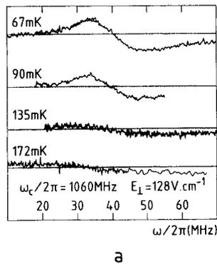
FIG. 2. Experimental traces of shear-mode resonance observed at fixed magnetic field  $\omega_c/2\pi = 1060$  MHz and pressing electric field  $E_{\perp} = 128$  V cm $^{-1}$  for a series of temperatures. Density  $n = 6 \times 10^7$  cm $^{-2}$ . The ordinate is the derivative of the absorption with respect to the pressing field  $E_{\perp}$ .
