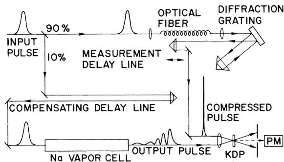
FIG. 1. Experimental arrangement used to measure the reshaped-pulse intensity.
