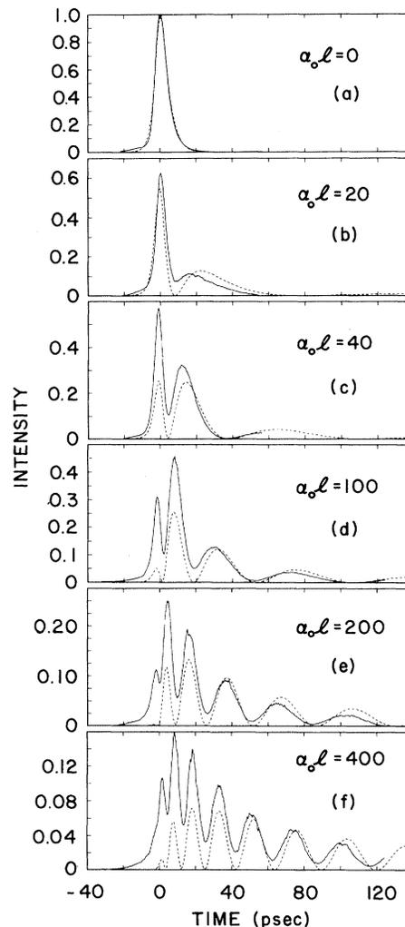
FIG. 2. Observed (solid curves) and theoretical (dashed curves) reshaped-pulse intensity after resonant propagation through sodium vapor of optical density  $\alpha_0 l$ . Theory is for transform-limited pulses tuned exactly to the Na absorption line and involves no adjustable parameters.
