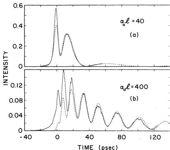
FIG. 3. Reshaped-pulse intensity, experiment (solid lines) and theory (dashed lines). Theory is for linearly chirped pulses with a triangular distribution of center frequencies consistent with the observed pulse spectrum.
