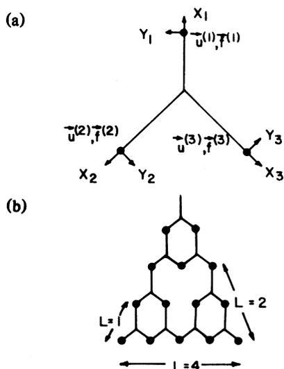
FIG. 2. (a) Three-terminal linear device representing an isotropic elastic material with arbitrary  $\lambda$  and  $\mu$ . At each terminal there is a displacement  $\vec{u}^{(i)}$  and a force  $\vec{F}^{(i)}$ ,  $i=1, 2, 3$ , and a local coordinate system  $(X_i, Y_i)$ . (b) Sierpinski-gasket-like  $L=4$  hookup of the unit elements of (a).
