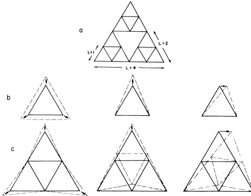
FIG. 1. (a) Sierpinski gasket in 2D with  $L=4$  unit cells to a side. Each bond corresponds to a simple spring with spring constant  $k_0$ . (b),(c) Three possible deformations of the  $L=1$  and  $L=2$  gaskets, respectively. Note that to order  $\delta L$ , only the external bonds change their lengths.
