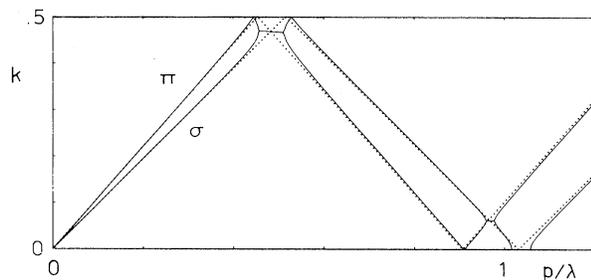
FIG. 1. Exact (solid lines) and approximate (dotted lines) dispersion curves.  $\epsilon_1 = \epsilon_2 = 2$ ,  $\epsilon_3 = 3$ ,  $\theta = 30^\circ$ ,  $\theta_i = 45^\circ$  in glass ( $n_i = 2.3$ ),  $p$  = helix pitch,  $\lambda$  = light wavelength,  $k = K_z/q$ . The approximate  $K_z$  values are given by Eq. (3); for the exact ones see Ref. 9.
