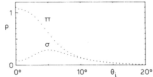
FIG. 2. Normalized differences between approximate and exact wave vectors vs  $\theta_i$  for  $\theta = 30^\circ$ ,  $p/\lambda = 0.6$ ,  $\epsilon_1 = \epsilon_2 = 2$ ,  $\epsilon_3 = 3$ ;  $\rho = \Delta K / (K_{1z} - K_{2z})$ , where  $K_{1z}$  and  $K_{2z}$  are the exact eigenvalues of Eq. (1) and  $\Delta K$  is the difference between the approximate and the exact eigenvalue of each eigenfunction.
