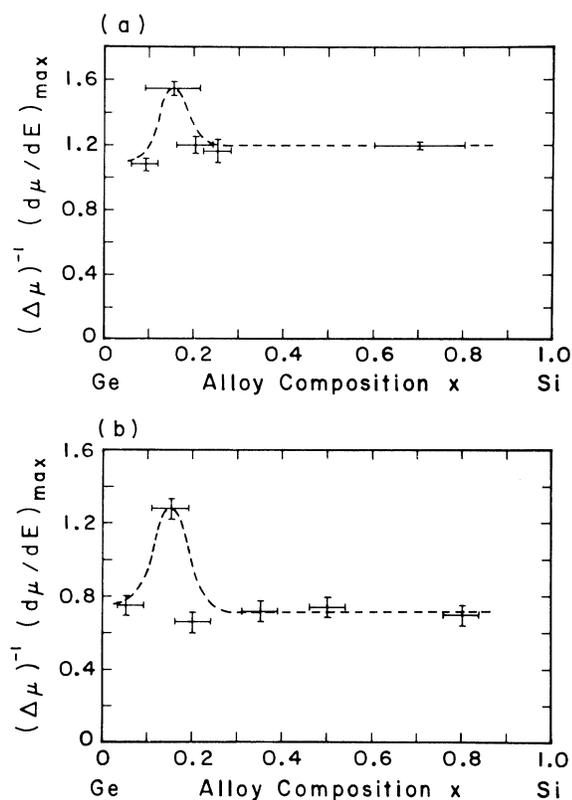
FIG. 3. Maximum normalized slope of the edge  $(\Delta\mu)^{-1}(d\mu/dE)_{\max}$ —the maximum energy derivative of the absorption at the  $L_3$  edge, divided by the absorption increase at the edge—as a function of alloy composition  $x$ , for (a) the transmission measurements, and (b) the electron-yield measurements. Note that different samples were used for the two types of measurements. The dashed line is a guide to the eye.
