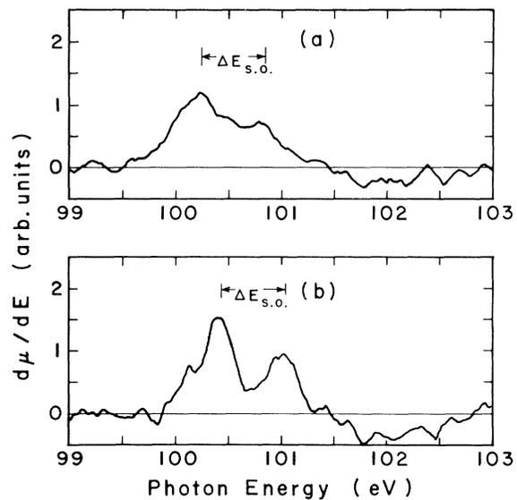
FIG. 2. The derivative of the normalized absorption coefficient  $d\mu/dE$  as a function of x-ray energy for (a)  $\text{Si}_{0.7}\text{Ge}_{0.3}$  and (b)  $\text{Si}_{0.15}\text{Ge}_{0.85}$ , determined in transmission. The spin-orbit splitting of the  $L_{2,3}$  edge is indicated as  $\Delta E_{s.o.}$ . The different spectra have been plotted with different vertical scales.
