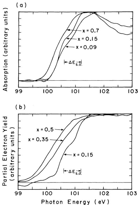
FIG. 1. Absorption coefficient  $\mu$  as a function of x-ray energy for several of the  $\text{Si}_x\text{Ge}_{1-x}$  alloys as determined in (a) transmission, and (b) electron yield. Data smoothing is described in Ref. 5. The spin-orbit splitting of the  $L_{2,3}$  edge is indicated as  $\Delta E_{s.o.}$ . Note the prominent shoulder evident for  $x = 0.15$  but not for other values of  $x$ . The different spectra have been plotted with different vertical scales.
