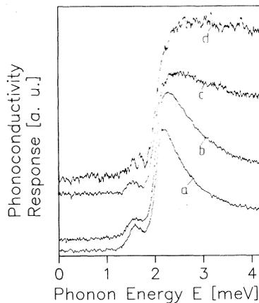
FIG. 2. PIC response signal for various illuminations, same sample as sample I of Fig. 1, and  $T=1.0$  K. Curve *a*, room-temperature radiation through a stainless-steel tube held at 300 K at the top of the cryostat; curve *b*, additional illumination by the fiber optic (room light); curve *c*, additional illumination by a bulb through the fiber optic; curve *d*, higher light intensity from the bulb, same curve as curve I of Fig. 1.
