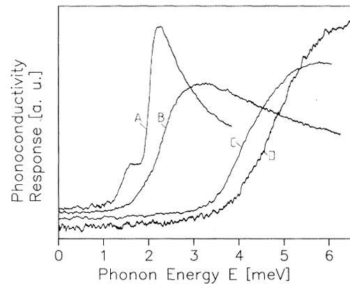
FIG. 3. PIC response signal for boron-doped silicon, all samples illuminated with the same light intensity, and  $T=1.0$  K. Curve *A*,  $[B]=5 \times 10^{13} \text{ cm}^{-3}$ ; curve *B*,  $[B]=9.5 \times 10^{14} \text{ cm}^{-3}$ ; curve *C*,  $[B]=5.4 \times 10^{15} \text{ cm}^{-3}$ ; curve *D*,  $[B]=9.0 \times 10^{15} \text{ cm}^{-3}$ .
