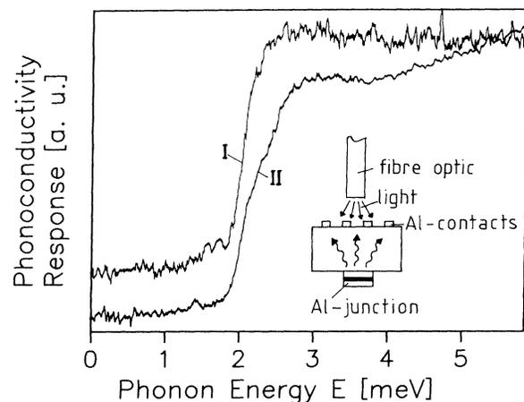
FIG. 1. PIC response signal for two different phosphorus-doped silicon samples at  $T = 1.0$  K. (I)  $[P] = 6 \times 10^{14} \text{ cm}^{-3}$ , (II)  $[P] = 6 \times 10^{15} \text{ cm}^{-3}$ .
