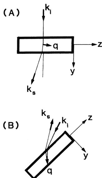
FIG. 2. Scattering geometries used. (a) Near forward scattering with the scattering vector ( $q$ ) nearly along the fiber axis ( $z$ ). (b) Near backscattering with the film tilted so that  $q$  lies about  $45^\circ$  from  $z$ .
