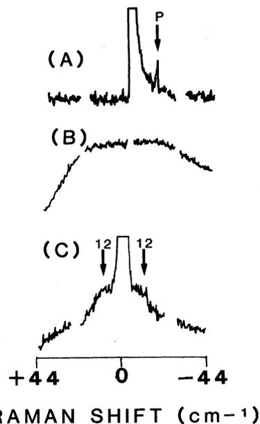
FIG.1. Performance of the tandem interferometer as a Raman spectrometer. The three spectra are (a)  $10\text{ }\mu\text{W}$  of the  $514.5\text{-nm}$  laser line fed into the spectrometer, (b) white light, and (c) a  $12\text{-cm}^{-1}$  LA mode in high-density polyethylene (the band center is marked with arrows). The  $13\text{-cm}^{-1}$  plasma line is labeled *P* on this and subsequent figures.
