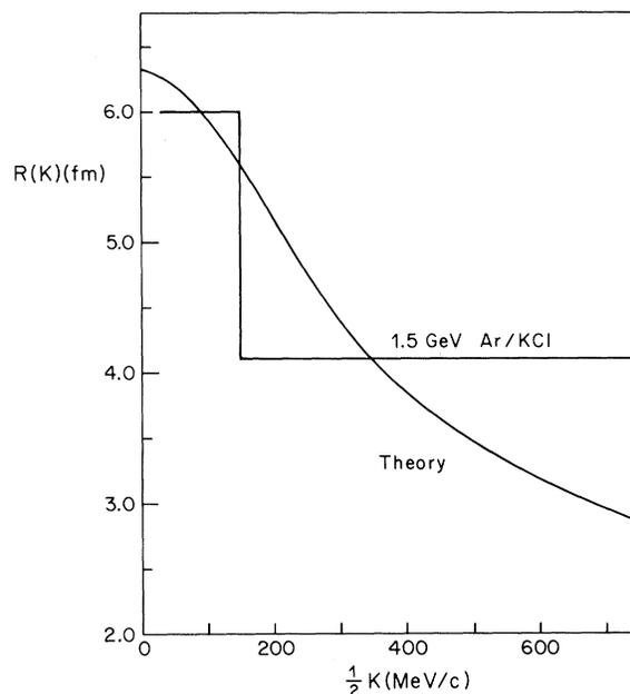
FIG. 2. The effective size of an expanding radial source with  $T/\gamma v = 100$  MeV and a radius of 7.75 fm is shown as a function of the total momentum of the two-pion pair. This is compared to experimentally determined values from 1.5-GeV Ar/KCl collisions where the effective source size was estimated for both pions having a momentum less than 150 MeV/c and for both pions having a momentum greater than 150 MeV/c (Ref. 7).
