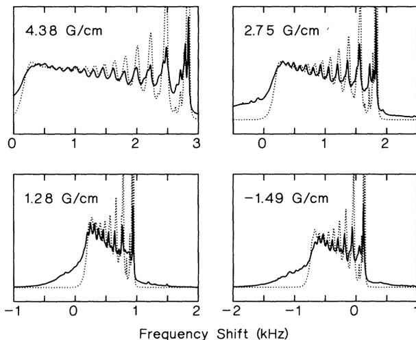
FIG. 1. NMR absorption at 2 MHz in normal liquid <sup>3</sup>He at zero pressure and  $T/T_c = 1.01$ . The vertical scale is different for each field gradient. Solid line is experiment; dotted line is theory. Experimental field shifts have been converted to equivalent frequency shifts with use of the <sup>3</sup>He gyromagnetic ratio.
