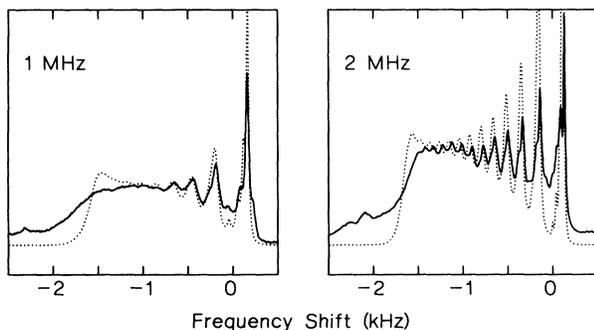
FIG. 3. Experimental (solid) and calculated (dotted) absorption line shapes at Larmor frequencies of 1 and 2 MHz. The field gradient is approximately  $-3.0$  G/cm for both cases.
