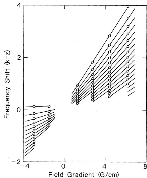
FIG. 2. Frequencies of the main series of spin-wave peaks as a function of field gradient, at a Larmor frequency of 2 MHz. Circles are experimental; lines are calculated.
