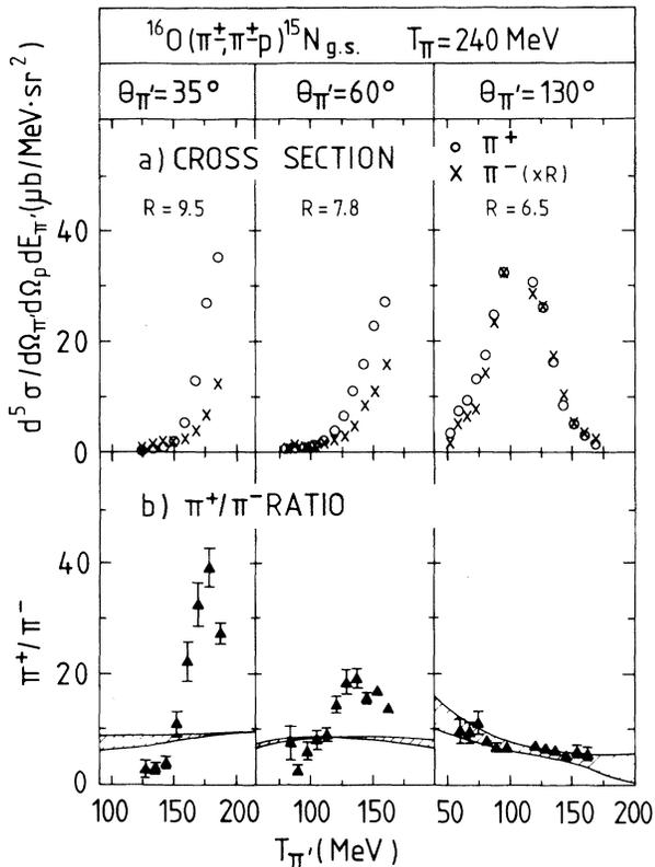
FIG. 2. (a) Differential cross sections for  $^{16}\text{O}(\pi^\pm, \pi^\pm p)^{15}\text{N}_{\text{g.s.}}$  for each pion angle, and for the full proton acceptance, as a function of  $T_{\pi'}$ . The  $\pi^-$  data are multiplied by  $R$ , the free  $\pi^+p/\pi^-p$  cross-section ratio. (b) Ratios of  $\pi^+$ - to  $\pi^-$ -induced cross sections for the conditions in (a); the hatched areas show the range of PWIA estimates using the initial- or final-state kinematics to define the interaction.
