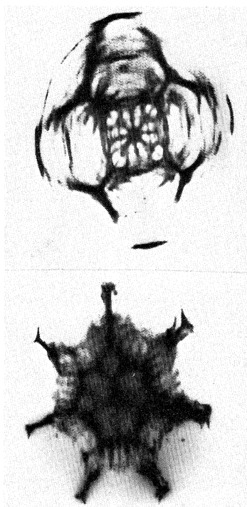
FIG. 1. Digitized optical intensity patterns for the (4,3) and (7,2) modes, respectively. The first index gives the number of angular maxima.
