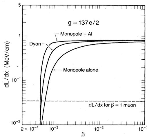
FIG. 1. Scintillation yield for monopoles in PS-10 acrylic scintillator as a function of velocity  $V = \beta c$ .
