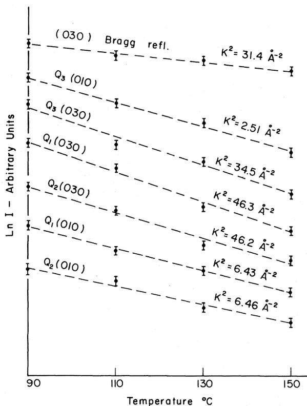
FIG. 2. Logarithm of integrated intensities of CDW satellites, and of the (030) Bragg reflections, vs temperature. Note the different  $K$  values for the satellite intensities. The  $(hkl)$  indices in parentheses are the Bragg reflections associated with each first-order satellite. The profiles have been arbitrarily shifted vertically for the sake of clarity.
