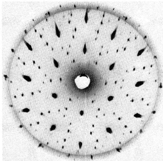
FIG. 1. Precession photograph of 1T-TaS<sub>2</sub> at 25 °C. ( $hk0$ ) planes. The heavy spots are the Bragg reflections; all other spots are second- and higher-order CDW satellites. Mo  $K\alpha$  radiation ( $\lambda = 0.71$  Å). Monochromator: flat graphite; 30 kV, 250 mA, 14.4 h. The streaks are due to incomplete monochromaticity.
