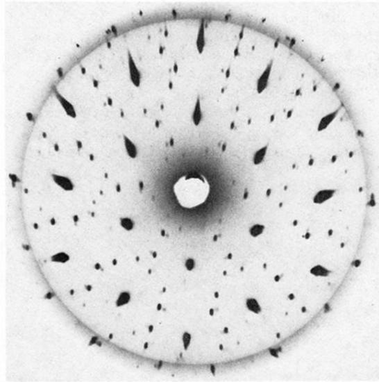
FIG. 1. Precession photograph of  $1T\text{-TaS}_2$  at  $25^\circ\text{C}$ . ( $hk0$ ) planes. The heavy spots are the Bragg reflections; all other spots are second- and higher-order CDW satellites. Mo  $K\alpha$  radiation ( $\lambda = 0.71 \text{ \AA}$ ). Monochromator: flat graphite; 30 kV, 250 mA, 14.4 h. The streaks are due to incomplete monochromaticity.
