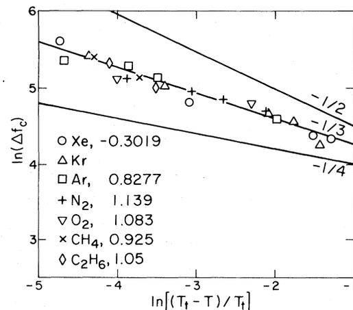
FIG. 3. Temperature dependence of the frequency shifts at critical thickness of type-2 films on Au(111).  $T_t$  is the triple point temperature of each adsorbate. For illustration, the data set for each gas was shifted vertically by a constant. The data are compared with power-law exponents  $-\frac{1}{2}$ ,  $-\frac{1}{3}$ , and  $-\frac{1}{4}$ .
