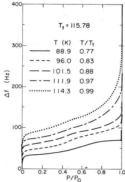
FIG. 1. Adsorption isotherms of Kr on Au(111) below its triple point. For clarity, successive curves have been shifted upward by 13 Hz.
