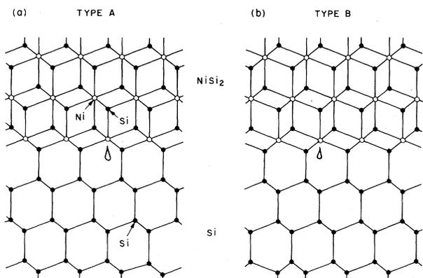
FIG. 2. Balls and sticks models of the two NiSi<sub>2</sub>-Si(111) interfaces viewed in the  $\langle 110 \rangle$  direction. Orbitals of unpaired electrons are also indicated.
