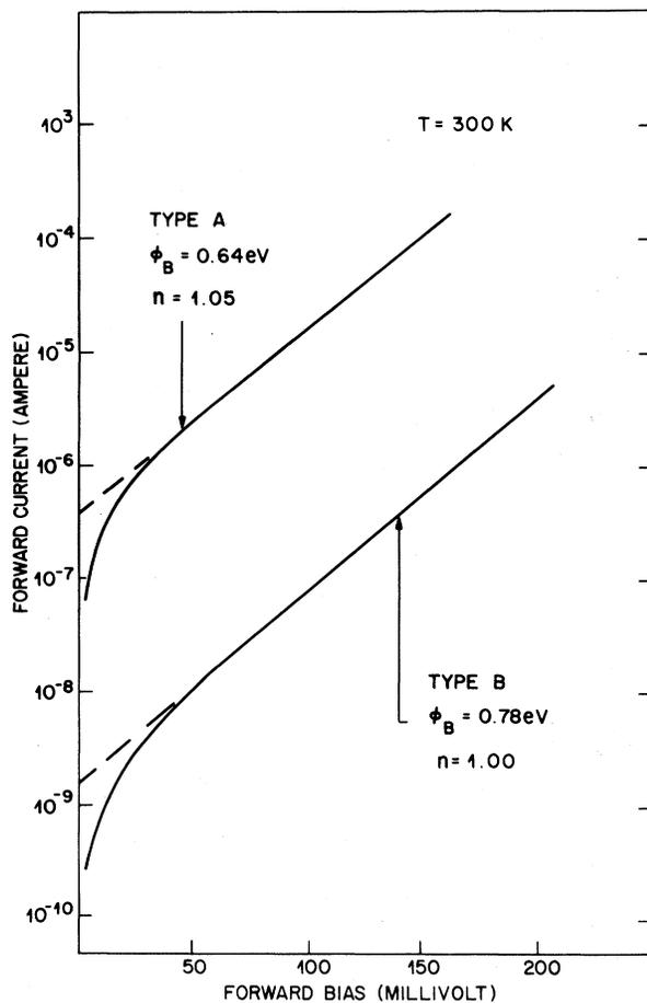
FIG. 1. Forward current characteristics of thin ( $\sim 70 \text{ \AA}$ ) type-A and type-B  $\text{NiSi}_2$  layers on  $\text{Si}(111)$ . Spot size is  $394 \mu\text{m}$ .
